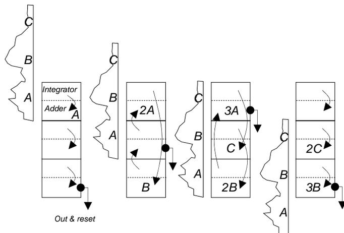
Fig. 6. Illustration of the Ajat CMOS TDI readout logic.
