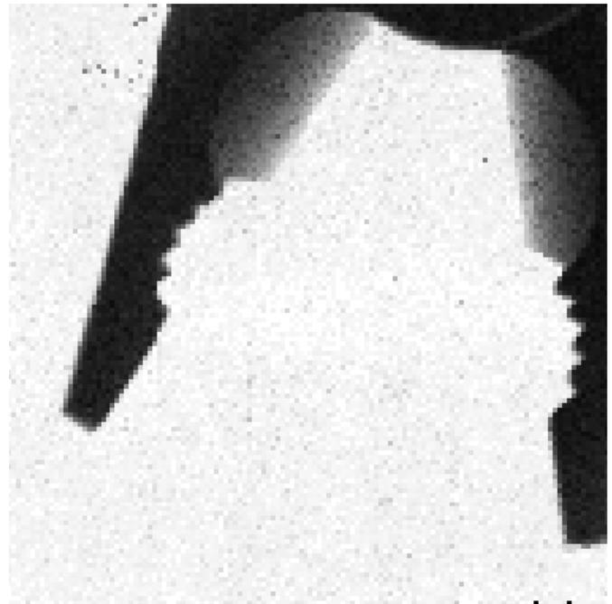
Fig. 13. A 90 kVp X-ray image of a workshop tool acquired with the PID proto camera. The area of the image is 4.4 x 4.4 cm<sup>2</sup>.
