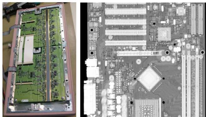
Fig. 7. An Ajat CdTe-CMOS TDI scanner (left) and an X-ray scan of printed circuit board (right) acquired at 10 cm/s with the TDI scanner.
