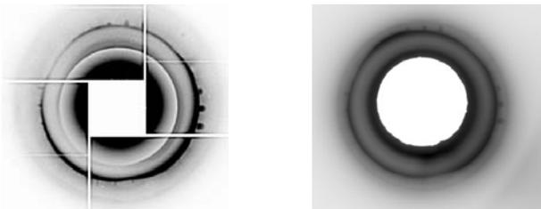
Fig. 2. Cross section X-ray images of a pipe, left: image acquired by the CdTe-CMOS camera and right: the corresponding film image [2].
