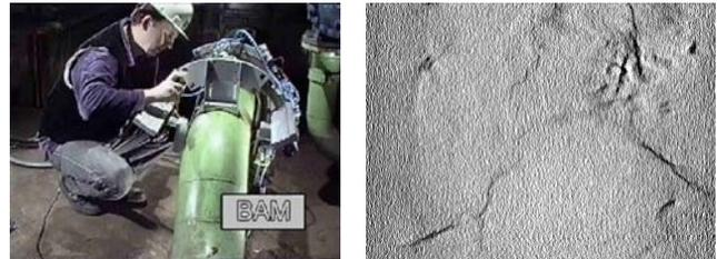
Fig. 3. The TOMOCAR imaging system by BAM (left) and an X-ray image of a welded joint acquired by the system with the Ajat CdTe-CMOS X-ray camera [2].
