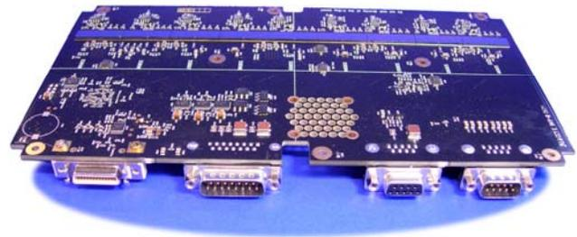
Fig. 4. An Ajat frame mode CdTe-CMOS X-ray scanner. The scanning slot has 9 hybrids giving a total slot length of 22.7 cm.
