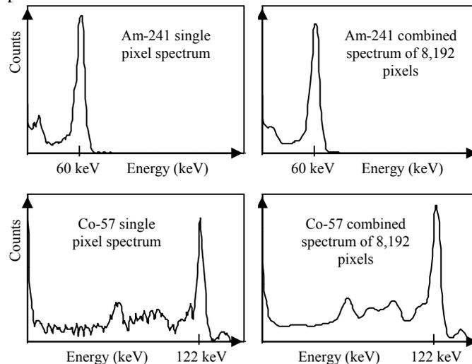
Fig. 10. Energy spectra of the PID.
