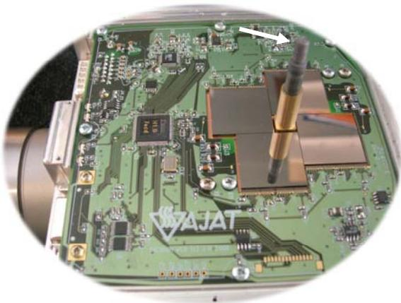
Fig. 1. A photograph of a small field of view CdTe-CMOS X-ray imager with a hole in the center of the active area.
