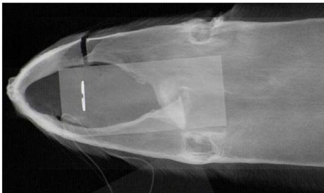
Fig. 8. An X-ray image of a mink fur acquired at 20 kV X-ray tube power with an Ajat TDI mode X-ray scanner (courtesy of Innospexion ApS, Denmark [3]).
