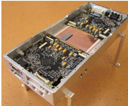
Fig. 9. The Ajat prototype PID camera. The photograph shows the camera with one CdTe-CMOS hybrid.
