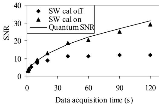
Fig. 11. The SNR of Am-241 images acquired by the PID proto camera.
